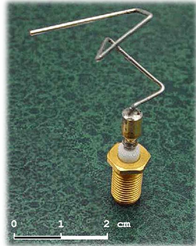
The 2006 NASA ST5 spacecraft antenna. This complicated shape was found by an evolutionary computer design program to create the best radiation pattern.
